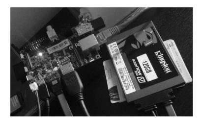
After a year of using a class10 SD card, I started to get some i/o errors... So decided to start taking advantage of one of the nicest features banana Pi has: SATA port + SATA power supply.
